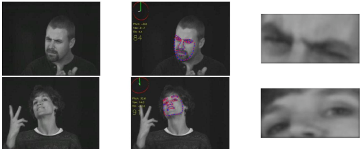
Figure 4. First column shows the input frame; second column the tracked face with the estimated 3D pose; third column the extracted eye and eyebrow region.
